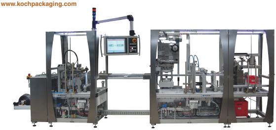
**Case/tray packers** The Axiom® IM Series case/tray packers feature next-generation electronic motion control technology. The product features an open design for convenience when cleaning and accessing machine components. New product sizes are easily added through the HMI and an electronic handwheel provides hand cycling when needed to
