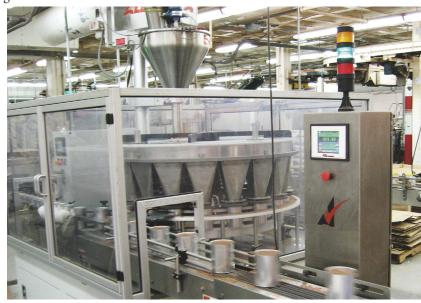
travel synchronously through the lower level. At the discharge of the starwheel, the scoops drop into the open tops of the canisters. A sensor at the inlet of the scoop feeder detects the presence or absence of canisters and turns the feeder on and off accordingly.
