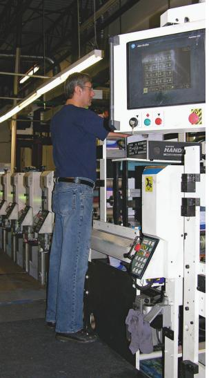
Packstar tests the PLA film on all of its lines, such as this Aquaflex press, to ensure that the substrate can be used on all its machinery.
