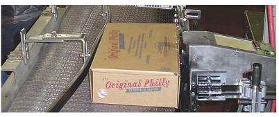
The printers provide variable data on up to 30 cases/min, or 12,000 cases/8-hr shift.
