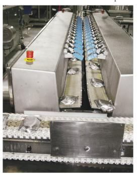
The MeadWestvaco cartoner requires very precise spacing of the pouches entering the machine, so Faribault installed two feeding machines. Each consists of a series of roller sections driven by computer-controlled stepper motors that are triggered by sensors that detect the gaps between the pouches and adjust the speed of the individual roller sections to separate the pouch according to the required spacing.
