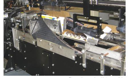
The pouches are placed in two parallel rows of five pouches each, all facing the same direction. Next, the two halves of the carton are folded together while retaining the pouches inside.
