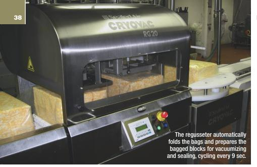
times. The machine door can be opened so that an operator can load the bags onto spreader plates, which are activated by a start/stop button on a control interface. A warning light on the door tells the operator that a bag cassette is about to run out of bags.
