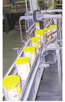
A diverter splits the flow of canisters to the two casepackers.
