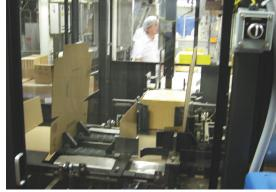
After the bag of cheese exits the regusseter, top, it is vacuumized for a snug fit and the block of cheese is case-packed, above, and palletized. The wraparound cases are erected, loaded and glue-sealed at a rate of about 12 blocks/min.
